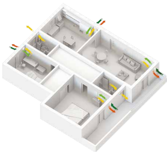
ALTERNATED SIMPLE-FLOW SYSTEM WITH STATIC HEAT RECOVERY.
