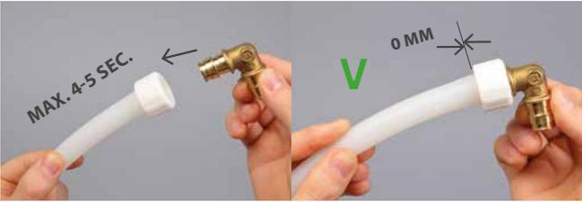
**FITTING INSERTION.** Before the pipe shrink back insert the GX fitting, pushing pipe and ring up to the fitting stop shoulder.
