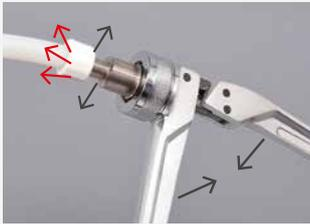
**EXPAND THE PIPE.** Select the proper expansion head and start gradually to expand the pipe.
