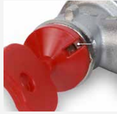
2. Set the R73PY010 key on the bonnet stem, fitting it in the only position allowed (letter "N" visible from the slot of R73PY010 key and facing the reference "A" on the valve body). Turn the bonnet stem using the key R73PY010 until the desired presetting number number appears from the slot of the key.
