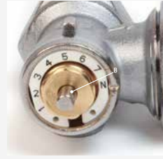
3. Remove the wrench R73PY010, the stem "B" will be on the desired pre-setting position, marked by the number on the valve ring. Adjustment positions 0,5 (single notch) - 1 - 2 - 3 - 4 - 5 - 6 - 7 - N (N = fully open).
